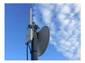
A mesh network is also self-redundant to the extent possible. The idea is to deploy many low-cost devices so there are several connections and paths to other nodes available.
